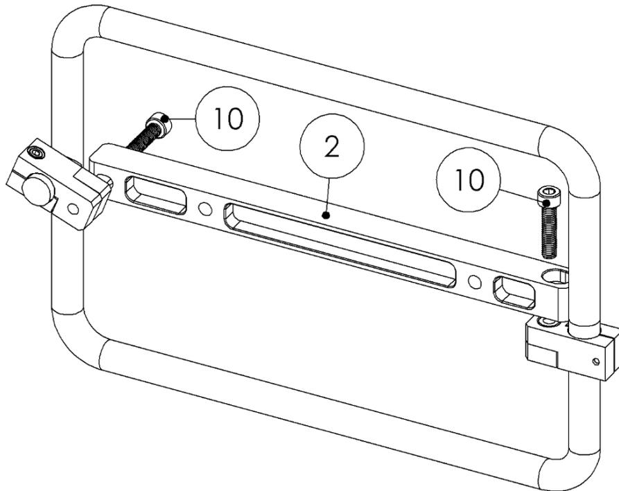
3. Install the Base and Top Bracket to the Main Mounting Strut using the M8x30 socket head cap screws.
