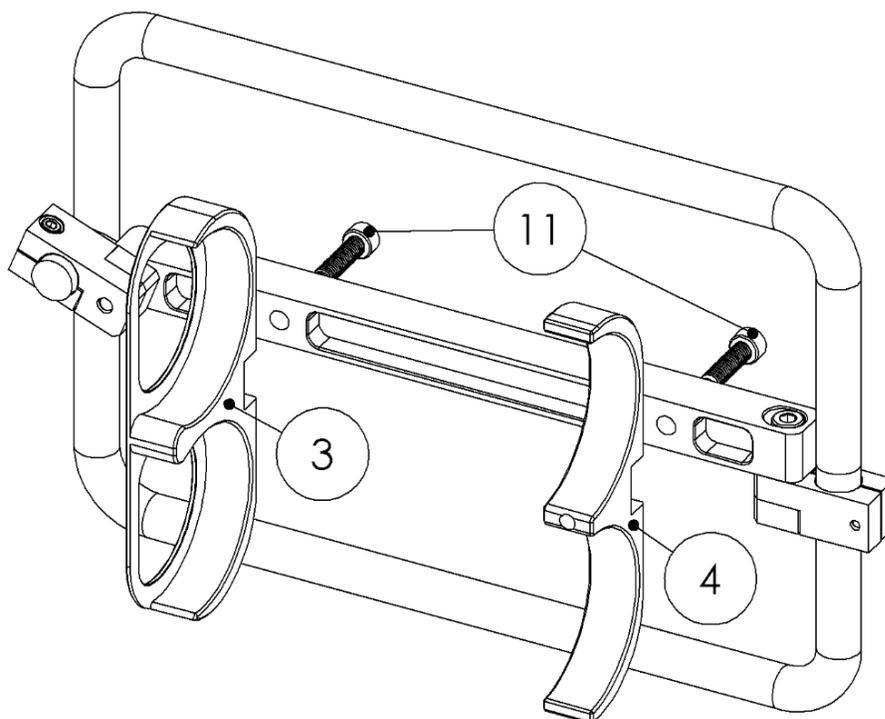
4. Install the Clamp and Quick Release Mechanism to the Top Bracket to complete the installation.
