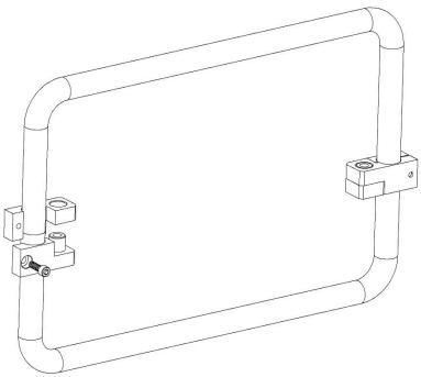
2. Install the Main Mounting Strut to the Pannier Mounting Split Clamps using the two M8X35 socket head cap screws. Using a measuring tape or ruler, align the Main Mounting Strut so that it is parallel and equidistant between the top and bottom horizontal tubes of the pannier mounting frame. Once aligned, tighten the M8 and M5 fasteners.
