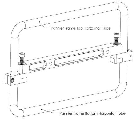
3. Install the Base and Top Bracket to the Main Mounting Strut using the M8x30 socket head cap screws.
